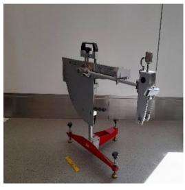
Figure 2 Testing Recoat Anti Slip Topcoat 14 days after application in escalator area
