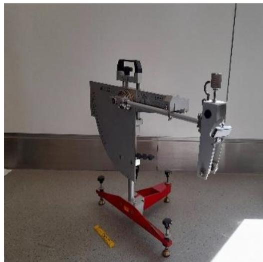
Figure 2 Testing Recoat Anti Slip Topcoat 14 days after application in escalator area
